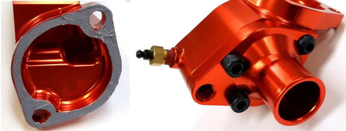
8. Using supplied sealant, apply a thin coat to main housing as shown in Fig C. Also apply to thermostat side of the main housing. You do not need to apply sealant to the thermostat housing. Just one side of that interface is sufficient.
