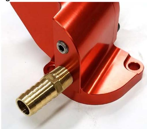
11. Install bleed nipple in top of housing, Fig D. Bleed nipple has pre-applied sealant and is 1/8 NPT tapered thread. It will naturally begin to bind as you rotate it in. Use only modest torque to avoid cracking housing.
