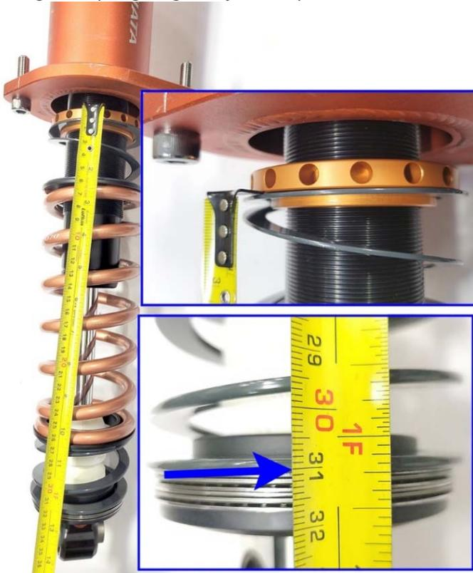
One full rotation on rear preload collar is roughly 2mm change in pinch weld height.
