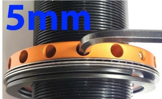
One full rotation on rear preload collar is roughly 2mm change in pinch weld height.
