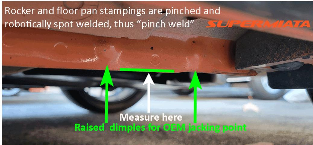
Typical pinch weld height adjustment range listed below, assuming a 24.3-24.7" tall tire. Exact range varies with weight of car and tire diameter.
